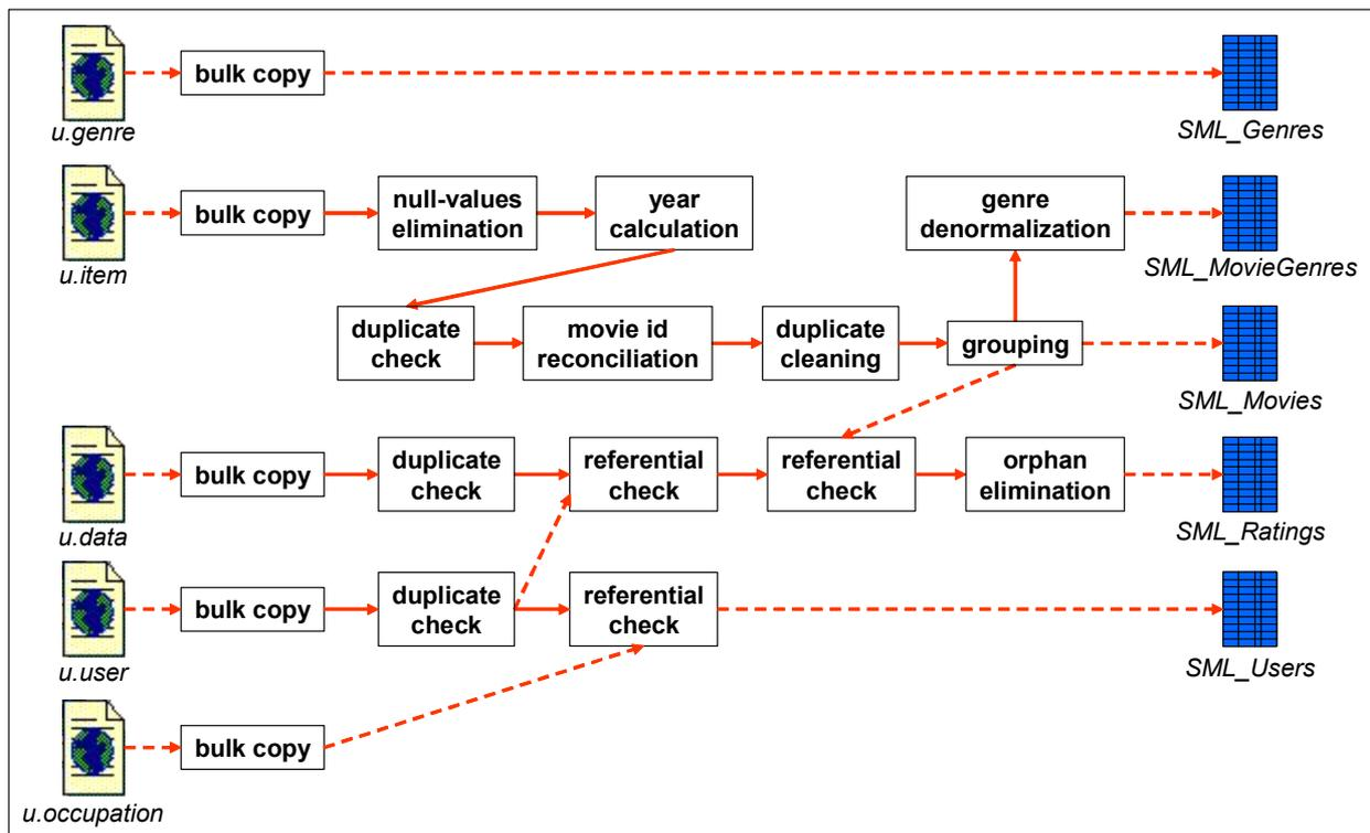
Figure 15 – ETL workflow for the small data set
