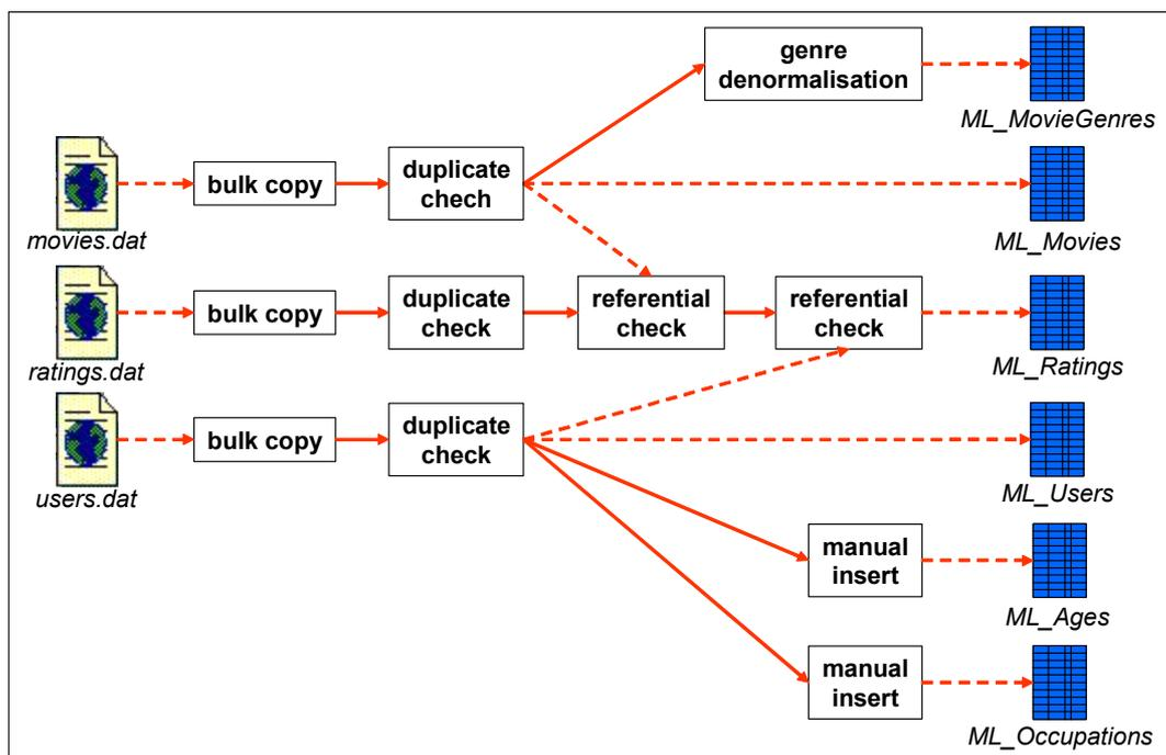
Figure 14 – ETL workflow for the large data set
