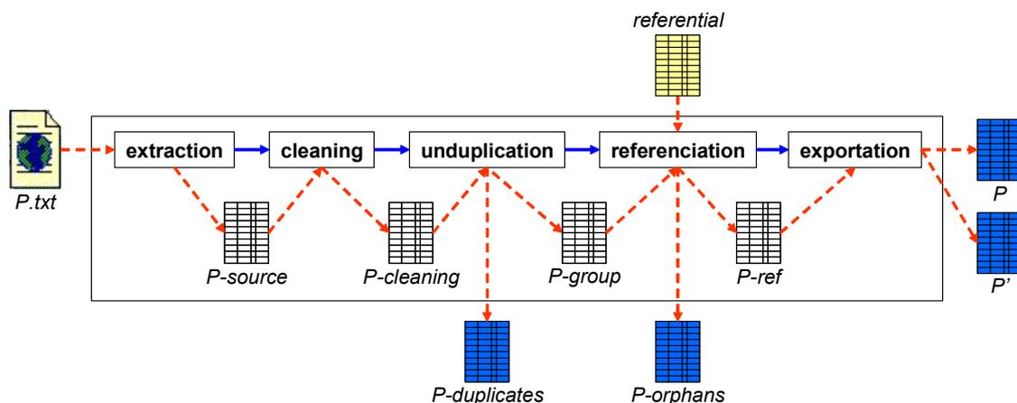
Figure 12 – High-level ETL process
